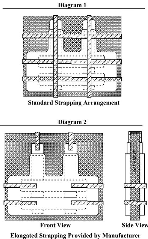
*Figure 8. Acceptable strapping methods*
